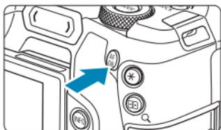
Has the same effect as pressing the shutter button halfway in **[Fv]**, **[P]**, **[Tv]**, **[Av]**, **[M]**, or **[BULB]** shooting mode.
