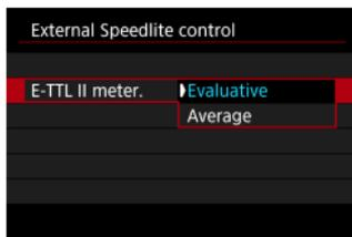
For normal flash exposures, set it to **[Evaluative]**. If **[Average]** is set, the flash exposure will be averaged for the entire metered scene. Depending on the scene, flash exposure compensation may be necessary. This setting is for advanced users.
