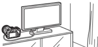
By connecting the camera to a television with an HDMI cable, you can play back the captured still photos and movies on the television. Using the HDMI Cable HTC-100 (sold separately) is recommended.
