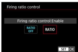
With a macro flash (MR-14EX II, etc.) compatible with flash function settings, you can set the flash ratio between flash tubes or flash heads A and B, or use wireless flash with additional receiver units.
