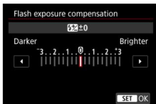
You can set flash exposure compensation up to  $\pm 3$  stops in 1/3-stop increments.
