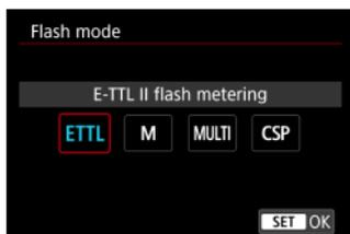
**[E-TTL II flash metering]** is the standard mode of EL/EX series Speedlites for automatic flash photography.
