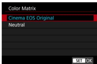
Using a color matrix, you can specify how colors are reproduced, to plan for postproduction processing.
