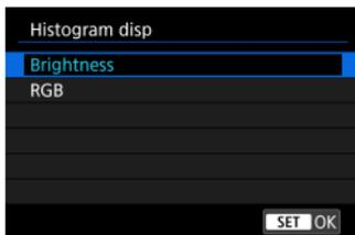
The brightness histogram shows the exposure level distribution and overall brightness. The RGB histogram is for checking the color saturation and gradation. You can switch the histogram displayed by pressing the <INFO> button when <INFO> is displayed in the lower left of the [**▶**3: Playback information display] screen.
