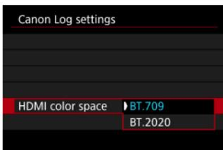
[**HDMI color space**] can be set when [**Canon Log**] is set to [**On (10bit)**] and [**Color Matrix**] to [**Neutral**]. Choose [**BT.709**] or [**BT.2020**] as the color space for HDMI output.
