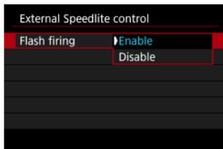
To enable flash photography, set to **[Enable]**. To disable flash firing or enable only the AF-assist beam, set to **[Disable]**.
