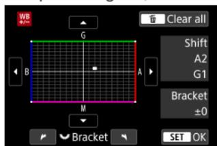
One level of the blue/amber correction is equivalent to approx. 5 mireds of a color temperature conversion filter. (Mired: Unit of measure for color temperature used to indicate values such as the density of a color temperature conversion filter.)
