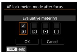
For each metering mode, you can set whether to lock the exposure (AE lock) after achieving focus with One-Shot AF by pressing the shutter button halfway. The exposure will be locked while you keep pressing the shutter button halfway. Checkmark [✓] the metering modes for when AE lock is to be applied. Select a metering mode []///, then press <SET> to append a checkmark [✓]. Select [OK] to register the setting.
