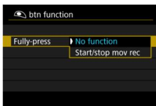
With [**Fully-press**] set to [**Start/stop mov rec**], you can start/stop shooting movies not only with the movie shooting button but also by pressing the shutter button completely or using Remote Switch RS-60E3 (sold separately, p.176).
