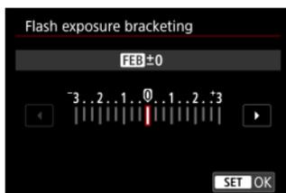
While changing the flash output automatically, three shots will be taken. For details, refer to the Instruction Manual of a Speedlite equipped with flash exposure bracketing.
