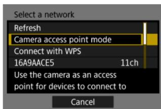
Camera access point mode is a connection mode for connecting the camera directly to each device via Wi-Fi. Displayed when [📶], [🖨️], or [📷] is selected in [Wi-Fi function].
