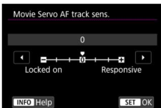
You can adjust the tracking sensitivity (to one of seven levels), which affects responsiveness if the subject strays from the AF point during Movie Servo AF, as when interfering objects move across AF points or when you pan.
