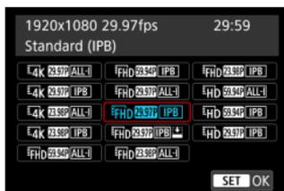
Under the **[📷 1: Movie rec quality]** tab, select **[Movie rec. size]** to set the image size, frame rate, and compression method. The movie will be recorded as an MP4 file.
