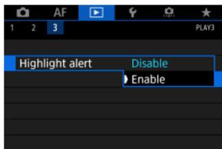
When [**▶ 3: Highlight alert**] is set to **[Enable]**, overexposed, clipped highlights will blink. To obtain more detailed gradation in the blinking areas where you want the gradation to be faithfully reproduced, set the exposure compensation to a negative amount and shoot again for a better result.
