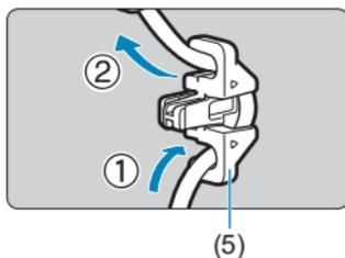
When using a genuine Canon interface cable (sold separately), run the cable through the clamp (5) as shown before attaching the clamp to the cable protector.
